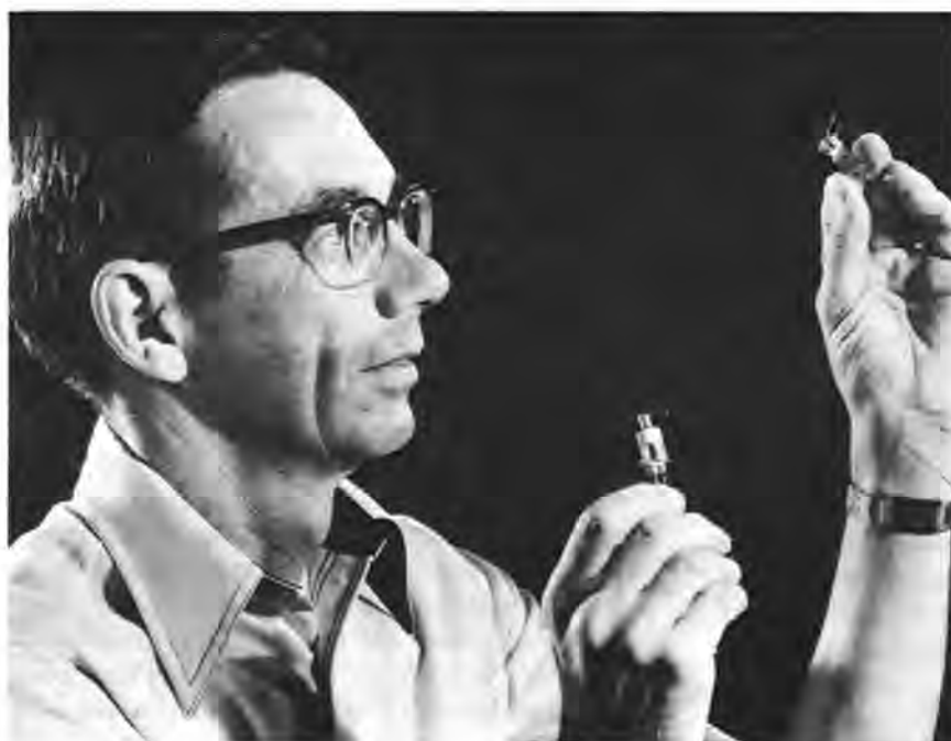
TWO SPRYTRONS are held by their inventor, Gordon Boettcher (DMTS, 2565). Used in a weapon to discharge capacitors for detonator firing and to switch pulse-forming networks, Sprytrons are rugged and radiation-tolerant. They replaced gas-filled switches, which underground nuclear tests showed could be triggered by the nearby detonation of an enemy's nuclear weapon.
